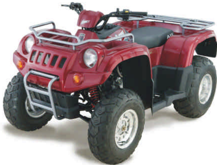
Multi-Purpose Front Rack with Three Independent Partitions
